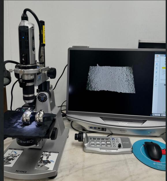
Figure 3. High resolution digital microscope used for non-contact surface roughness measurements..
