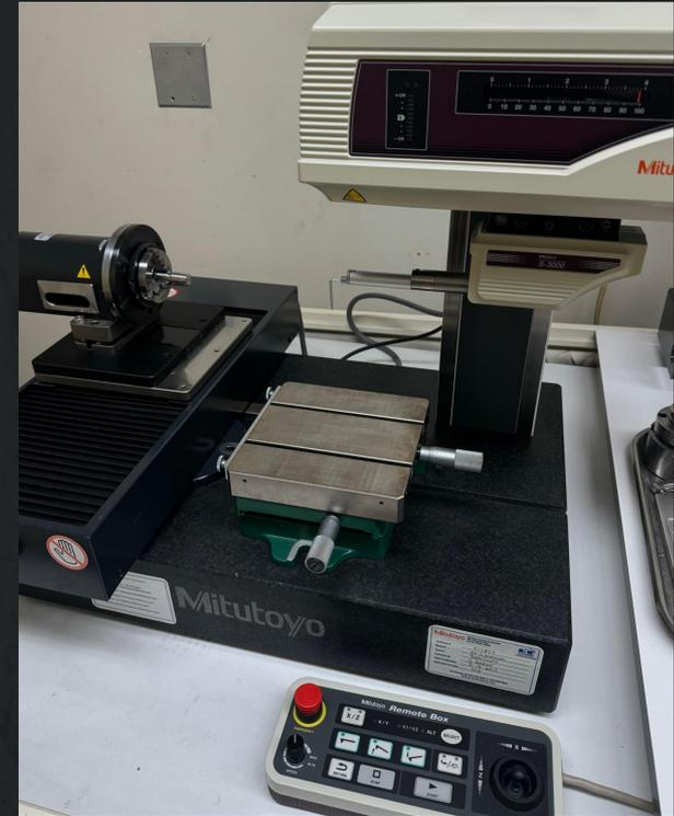
Figure 2. Contact profilometer used for surface roughness measurements..
